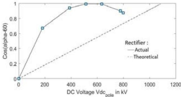
**Fig. 5 :** Theoretical and actual relation between  $\cos(\alpha - 60^\circ)$  and  $V_{dc\_pole}$  for rectifier during OLT
