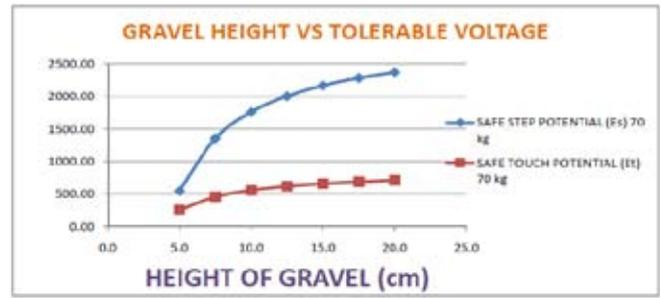
**Fig. 9 :** Impact of Height of Gravel on Safe Potentials (70 kg)
