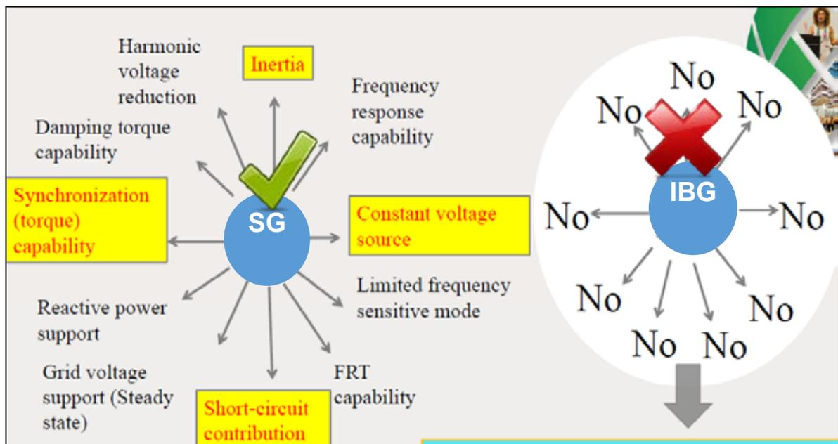
Fig. 3 : Characteristics Difference between SG and IBG
