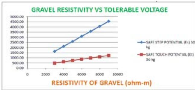
**Fig. 8 :** Impact of Resistivity of Gravel on Safe Potentials (50 kg)
