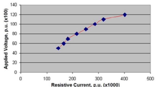
Fig. 6 : Variation of resistive component of leakage current with respect to applied voltage
