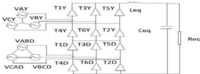
Fig. 11 : Schematic diagram of 12 pulse bridge ac to dc converter in open loop condition
