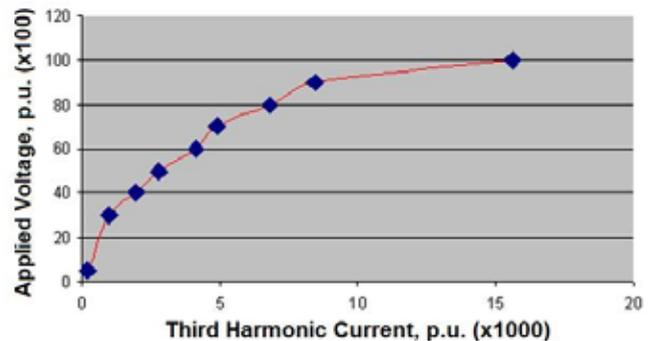
Fig. 5 : Variation of third harmonic component of leakage current with respect to applied voltage
