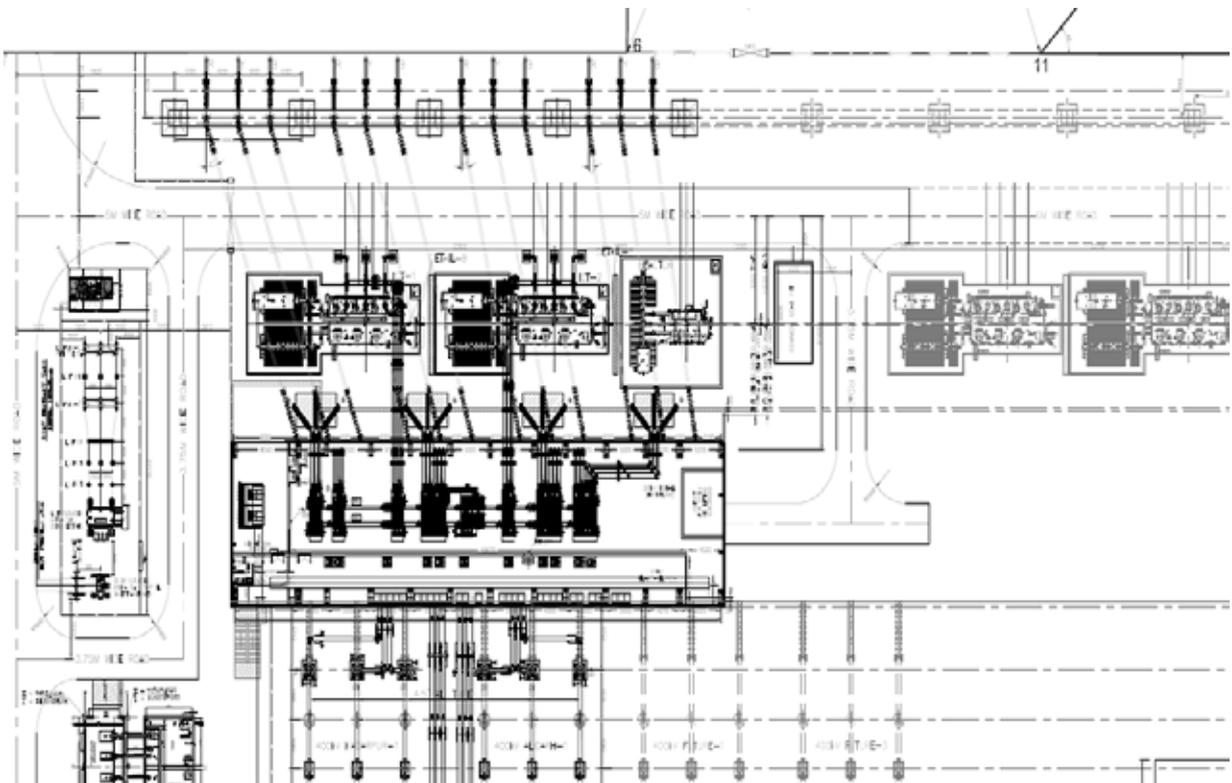
Fig. 3 : 220kV GIS Building (First Floor) Layout
