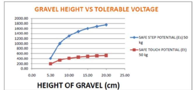
**Fig. 10 :** Impact of Height of Gravel on Safe Potentials (50 kg)
