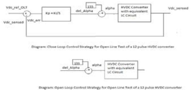
**Fig. 6 :** Closed and Open Loop control strategy for Open Line Test of a rectifier
