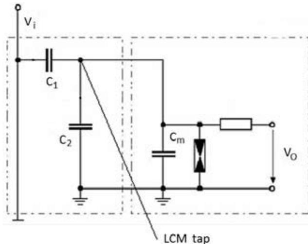
**Fig. 1** : Conventional Leakage Current Measurement Set-up
