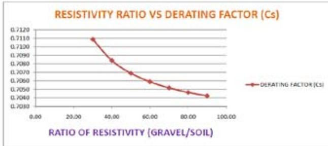
Fig. 11 : Impact of Resistivity of Gravel on Derating Factor
