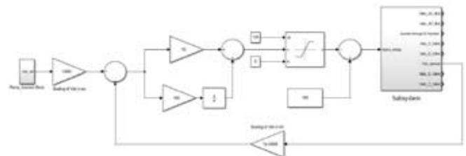
**Fig. 7 :** Closed loop control model in MATLAB Simulink
