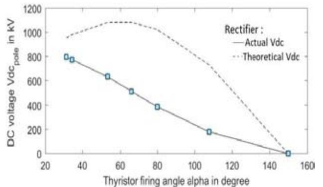
**Fig. 4 :** Theoretical and actual relation between  $Vdc_{pole}$  and  $\alpha$  for rectifier during OLT
