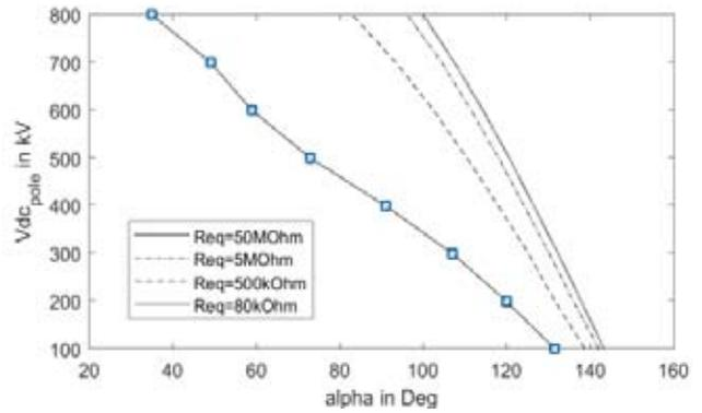
**Fig. 23 :**  $V_{dc\_pole}$  with respect to  $\alpha$  in degree during OLT for different  $Reg$
