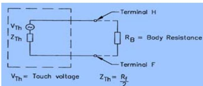
Fig. 4 : Thevenin Equivalent of Circuit of figure 3
