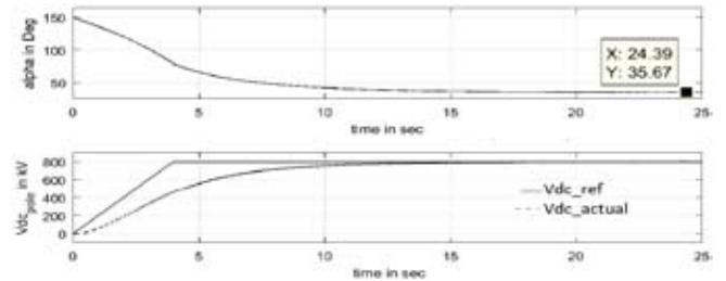
Fig. 17 : Closed loop simulation of rectifier(+ve pole) with circuit configuration 3 (c). DC Voltage command=800kV
