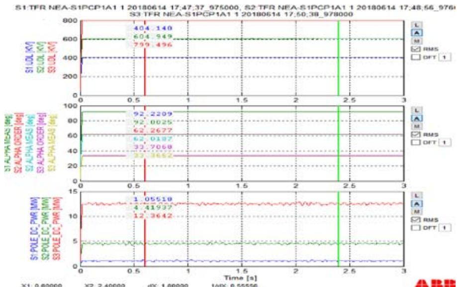
Fig 18 : Three sets of data (S1, S2, S3) for different reference voltages of 400 kV, 600 kV, 800 kV during Open Line Test operation of +ve pole at rectifier station 1.
