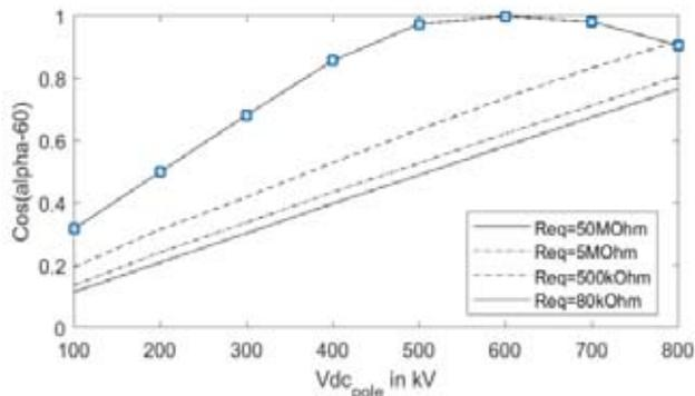
**Fig 22 :**  $\cos(\alpha - 60^\circ)$  with respect to dc pole voltage,  $V_{dc\_pole}$  during OLT for different  $Reg$ .
