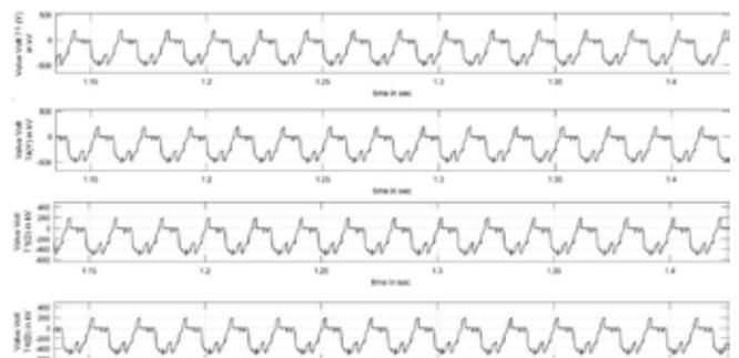
Fig. 12 : Voltage across the valves in first leg
