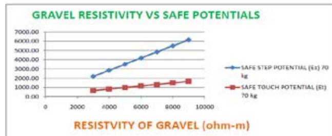
**Fig. 7 :** Impact of Resistivity of Gravel on Safe Potentials (70 kg)
