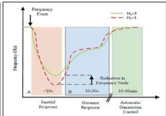
**Fig. 9 :** Frequency response spectrum & impact of Inertia on ROCOF
