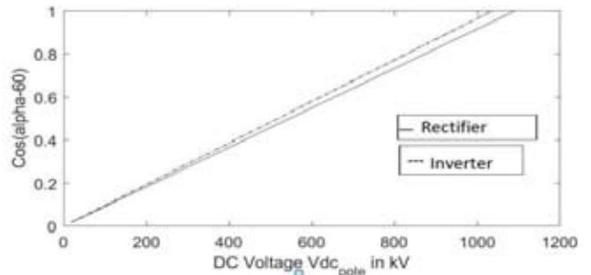
**Fig. 2 :** Theoretical relation between  $Cos(\alpha - 60^\circ)$  and  $Vdc_{pole}$  during normal power flow operation
