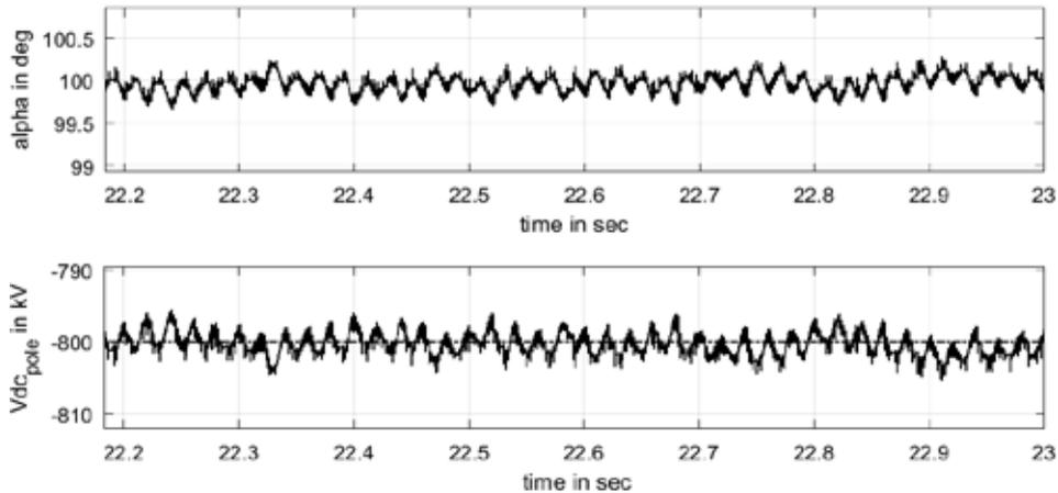
**Fig. 19 :** Closed loop simulation of (-vepole) of Station 2 with circuit configuration 3(a). DC Voltage command = -800 kV
