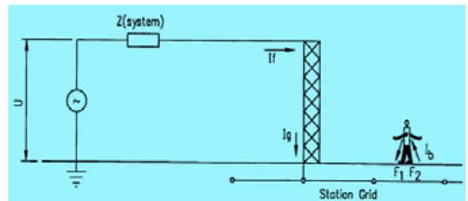
Fig. 5 : Different Resistances of Circuit for Step Voltage
