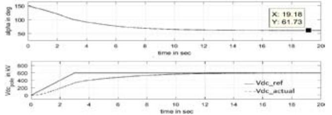
Fig. 16 : Closed loop simulation of rectifier(+ve pole) with circuit configuration 3 (c). DC Voltage command = 600 kV
