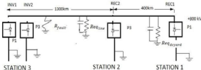
**Fig. 1 :** Equivalent Impedance model of Open Line Test (Rectifier Converter of Station 1 is connected to DC line with DC filter)
