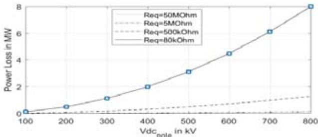
**Fig. 21 :** Theoretical dielectric loss with respect to dc pole voltage during Open Line Test for different equivalent resistance  $Reg$  (1)
