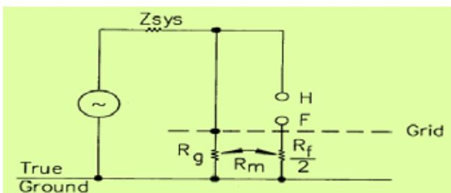
Fig. 3 : Different Resistances of Circuit for Touch Voltage
