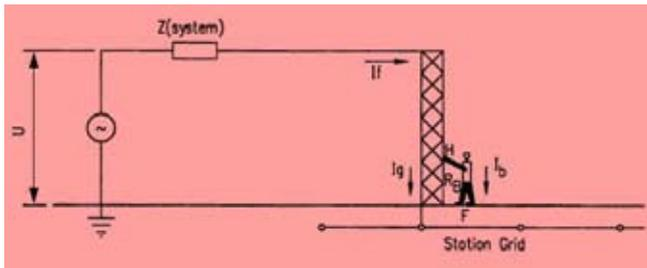
Fig. 2 : Flow of Current through the Working Staff during Fault
