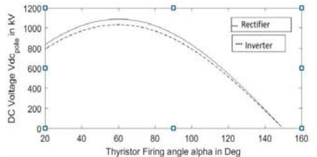
**Fig. 3 :** Theoretical relation between  $Vdc_{pole}$  and  $\alpha$  during normal power flow operation
