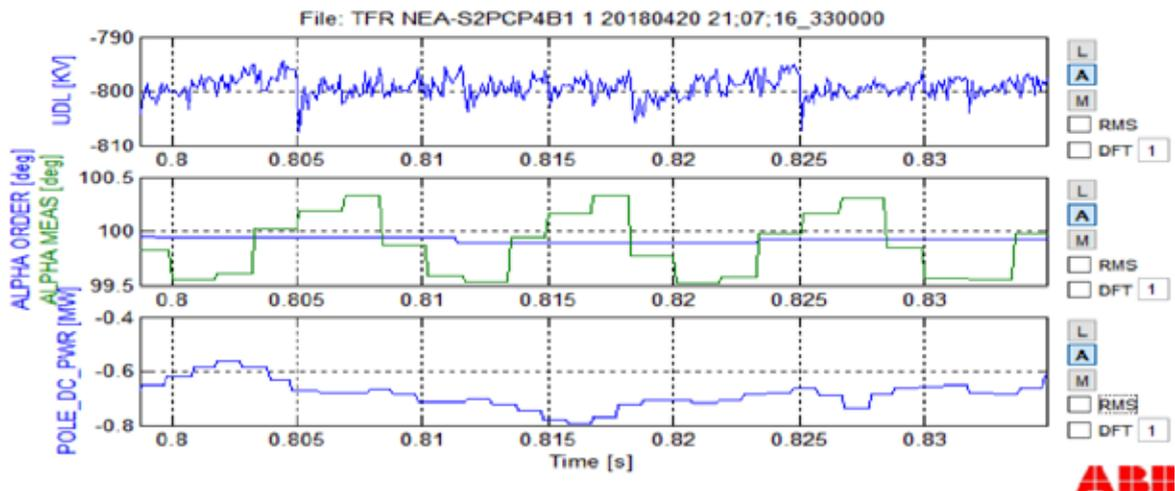
**Fig. 20 :** Negative pole of Station 2 with circuit configuration 3(a). DC Voltage command = 800 kV without considering the sign.
