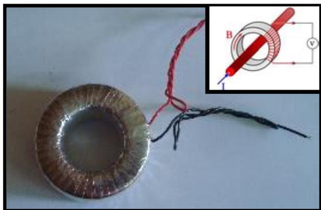
Fig. 2 : Typical Leakage Current Sensor developed in study
