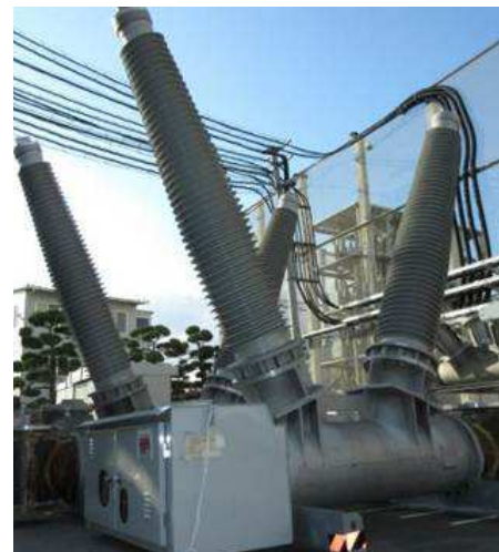
Fig. 9 : Prototype 420 kV GCB under interruption test
