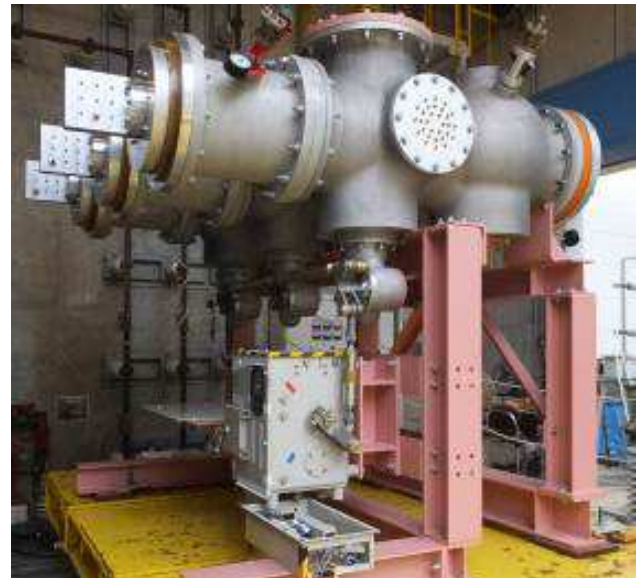
Fig. 8 : Prototype 420 kV GIS under short-circuit making test
